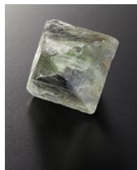
Fluorite, which has low refraction and color aberration, is used as the lens material.
