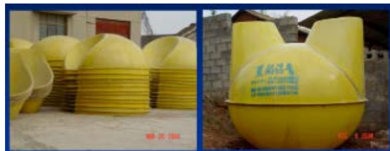
Commercialized digesters made of reinforced plastic with fiber glass
