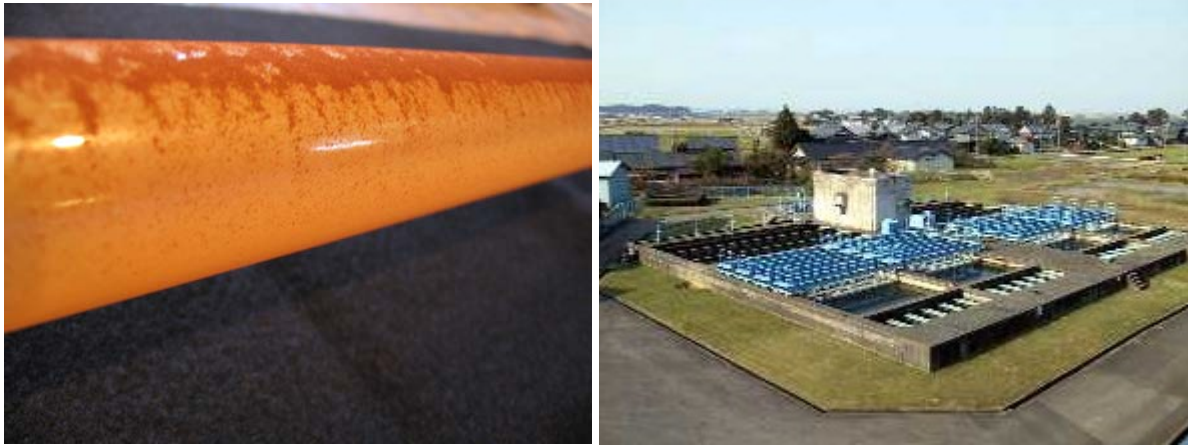
Figure 3. Examples of chemical precipitation processes. Left image: accumulation of Fe-based precipitant at a quartz:water interface in an ultraviolet (UV) photochemical reactor. Precipitation in this form can virtually occlude all UV radiation, thereby adversely affecting reactor performance. Right image: reactor system used for metal removal from water by chemical precipitation. The principles that govern the dynamics of these processes are also relevant to many other applications, including: softening, Fe and Mn removal, solidification/stabilization, and separation (recovery) of heavy metals.
