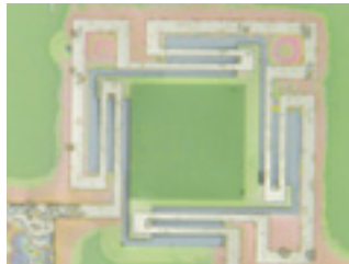
Photonic crystal filter (1000x)
