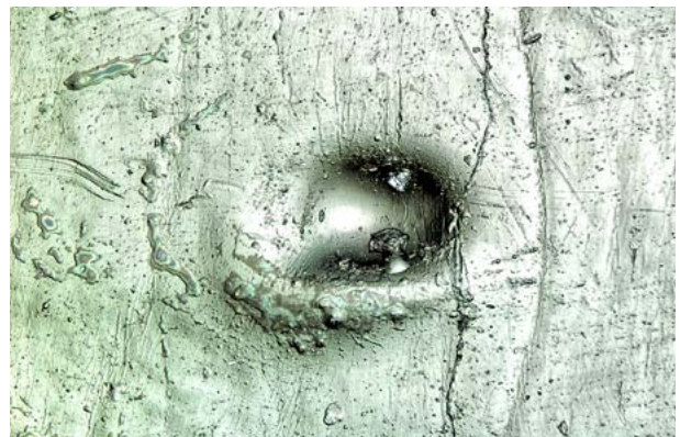
Light guide panel: Area and volume measurement (3000x)
